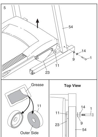
6. See the left inset drawing in step 5. Identify the outer side of the remaining Frame Spacer (11).
